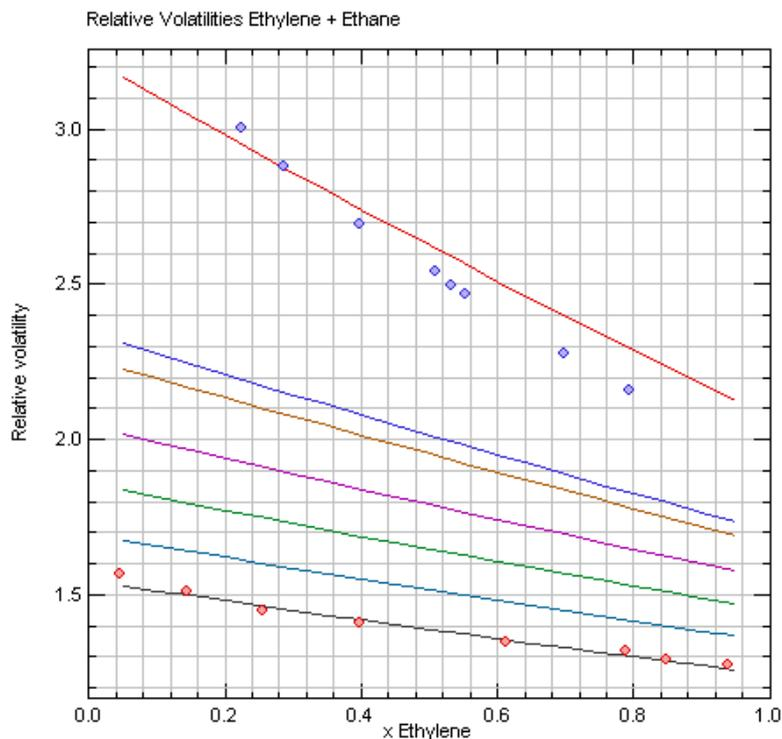
In case you are wondering why there are only two sets of relative volatility data when we see seven sets of VLE data, it is because only two of the data sets are complete sets of  $pxy$  data. The others are  $px$  data sets which don't allow the computation of relative volatilities (neither from  $py$  data).
