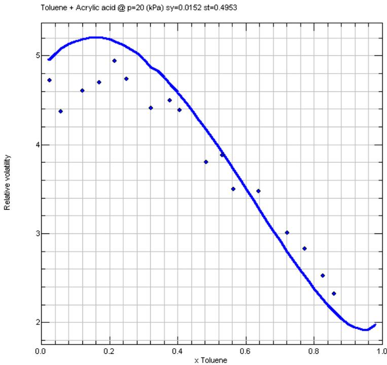
You can see that at high Acrylic Acid mole fractions, the relative volatility has a maximum whereas at high Toluene composition it has a minimum. It is also possible to display multiple sets of data on the phase diagram as well as on the parity plots, thereby making very easy a comparison of data and the model to verify that the selected model sufficiently well describes the VLE. Below is an example for the Ethylene and Ethane binary:
