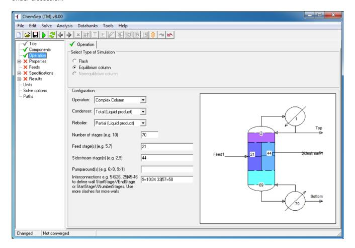
This action will create a new *Interconnections* panel to become visible. This is where we specify the vapor and liquid flow splits.
