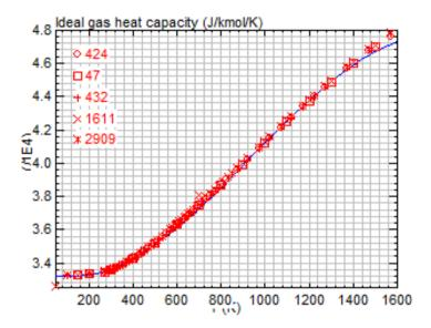
On occasion, however, it is necessary to evaluate the heat capacity at temperatures outside the valid range of the ChemSep correlations. Here is what happens if we extrapolate that correlation to 5000K.
