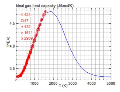
Clearly, not a correct extrapolation. (We should note that this is very far beyond the range at which any two-phase separation would be possible, so at these high temperatures we are dealing only with gas phases. That said, it remains possible that in a process flowsheet it might be necessary to evaluate the ideal gas heat capacity at temperatures outside the valid range.
