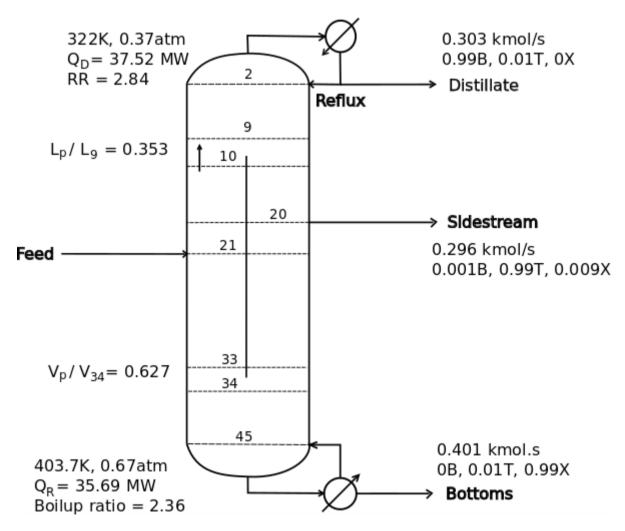
Before starting ChemSep, the first thing we should work out is the column stage numbering. This is an important step when creating an equation-oriented model. Based on the figure above, this column has 9 stages in the top section (the condenser is treated as a stage), 24 stages in each section beside the dividing
